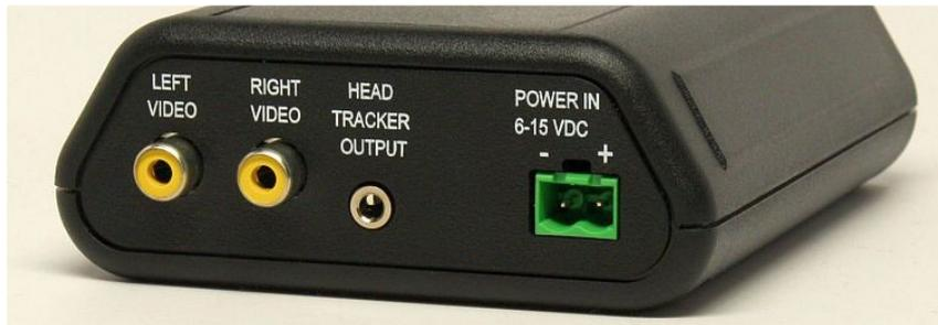
**Left and Right Video Inputs; Head Tracker Output; Power Input**
